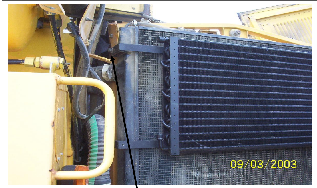
Condenser frame mounts to existing holes on the radiator frame
